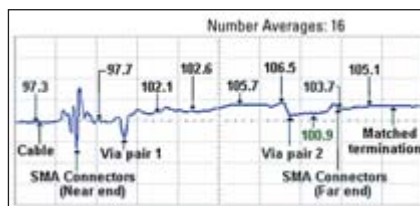
FIGURE 6. The DUT signature (differential impedance values in ohms) generated utilizing the normalized response.
