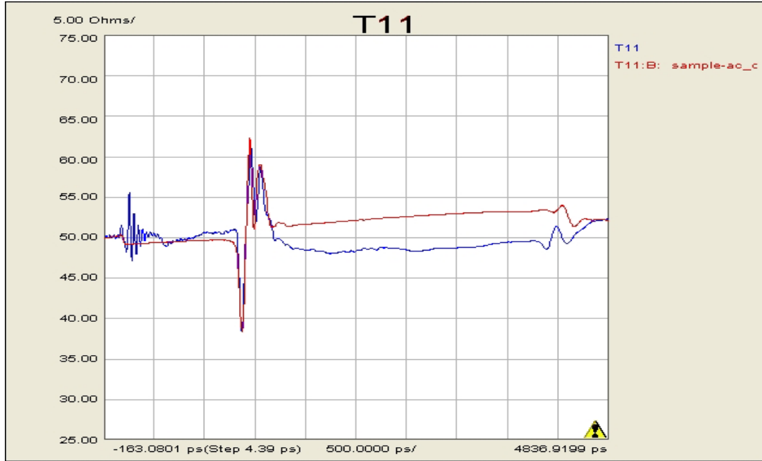
Figure 1: Measured and Simulated Z(t) Short Path.
