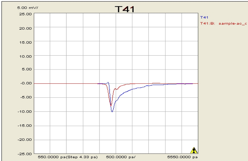
Figure 9: Measured and Simulated Far End Crosstalk - Short Path
