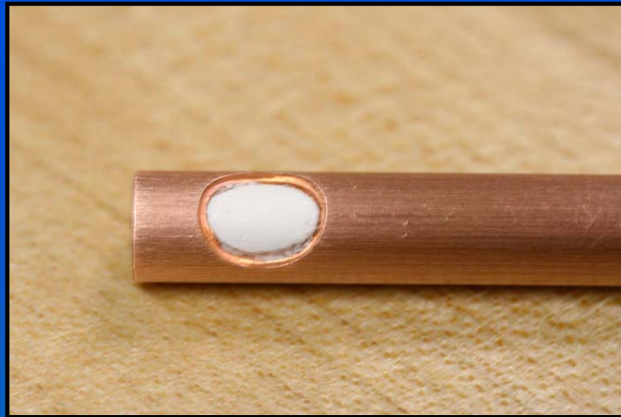
0.25" diameter semi-rigid cable with 0.25" diameter aperture
